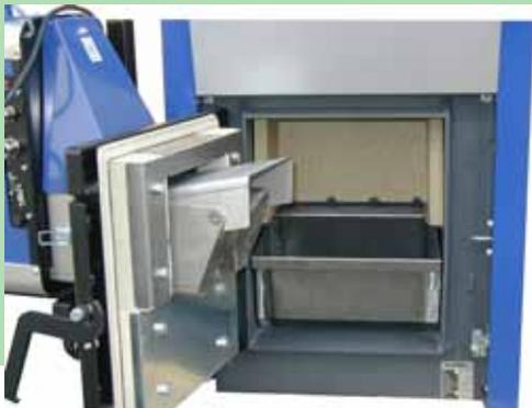
The main heat exchanger of the Compact is plain and build in vertically. Because of this dust can not stick easily to its surface. We have moveable turbulator sheets in it. These sheets can be moved up and down by a lever on the side of the boiler. By moving the sheets the surface of the heat-exchanger will be cleaned.
